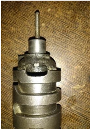
(B) Modified gear shifter drum. Fig. 6. Gear Position Sensor Arrangement.
