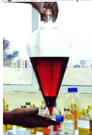
Fig 5. Settling of Biodiesel and Glycerine
